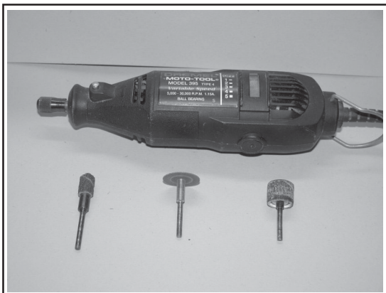
Figure 4: Dremel Tool with sanding drums and cutting disc.
