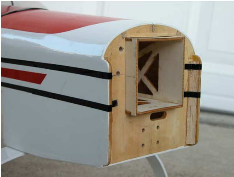
Battery Box Mounted in Firewall cut out Battery is accessible through wing saddle
