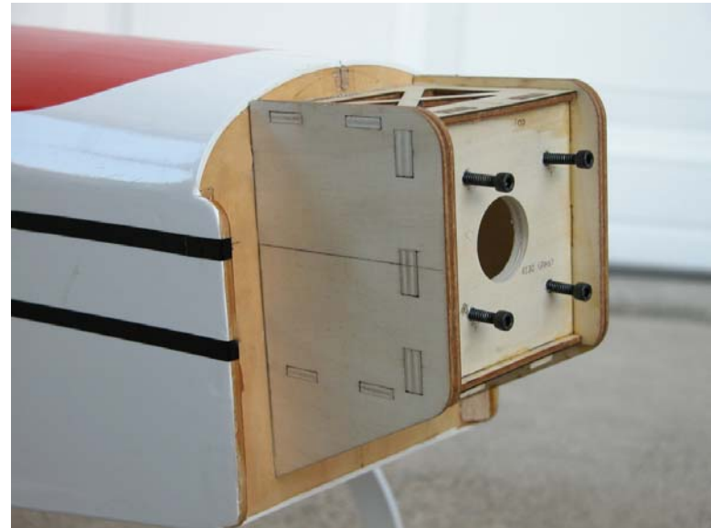
Motor mount Slips over Battery box and Secures to battery box and Firewall
